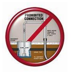
Connecting sump pumps to the Public Sewer is ILLEGAL If your sump pump is frequently operating, rain may have caused the groundwater to rise and flow into the sump pump pit. In some cases, the groundwater may remain high and cause the sump pump to run continually.
