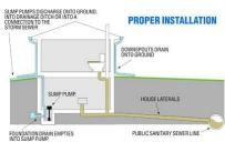
Sump pump discharge hoses may be connected to the **stormwater** system in the street. Residents MUST FIRST contact the town DPW or DOT for permission and guidance.
